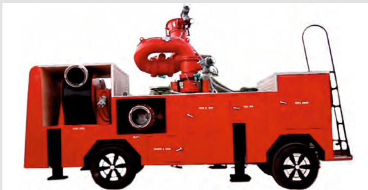
Trailer Mounted 10500 US GPM Foam Monitor with long dia hose
